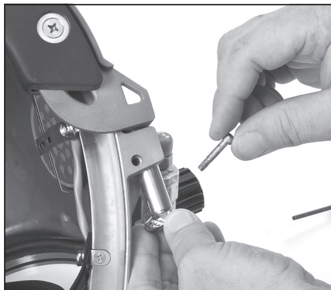
The screws that secure the sealed pulled pins must be properly installed and tightened.
