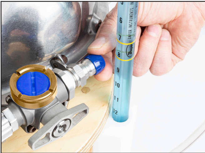
9) Ensure SBV is in open position (parallel).
