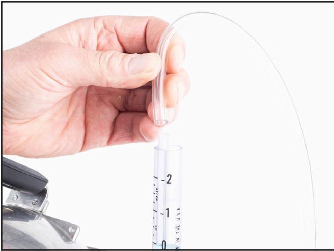
8) Cap Exhaust Hose Adapter fitting.
