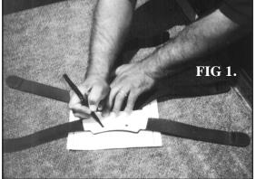
5) Place the spider with the EXO lettering facing UP, on top of the alignment template and press it flat so the curved edge lines up with the template. Place the hole marking template on top of the spider, again aligning the curved edge. Mark the hole position, FIG 1.
