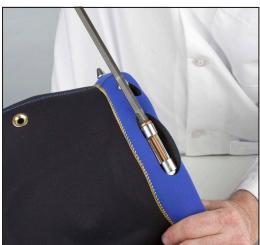
2. Use the bronze band adjustment screws, included in this kit, and start the screws a few threads—just enough to hold the bands together.
