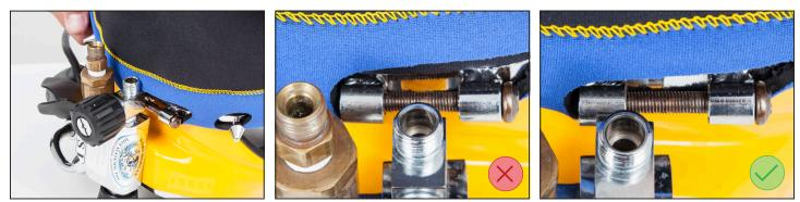
Make certain the bands are over the rubber of the molded face seal and the neoprene has NOT folded over the rubber.
