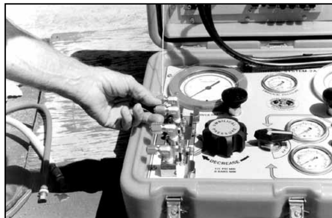
Figure 10 All of the outlet fittings on the KMACS 5 must be capped prior to storage.
