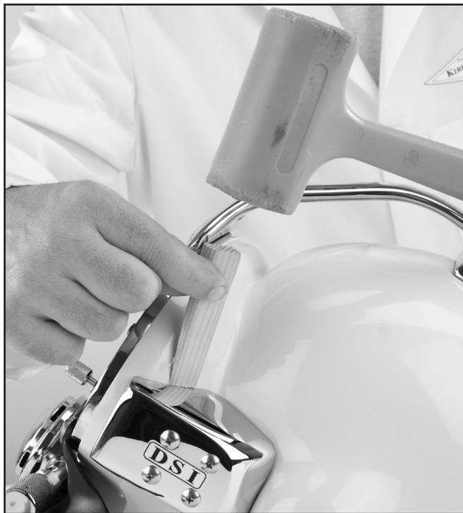
*Use a wooden wedge and the mallet to break the seal between the weight and the helmet shell. **DO NOT USE A SCREWDRIVER OR CHISEL TO REMOVE THE WEIGHT.** This could damage the helmet shell, requiring expensive repair.*
