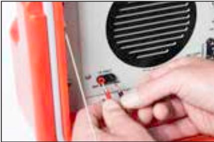
Match the Red and Black probes to the Red and Black receiving holes on the lower left panel of the communicator to connect the charge to the MK3-KMDSI communicator.
