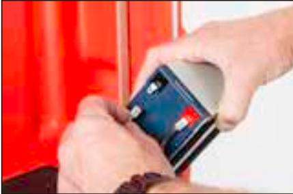
The battery is held in place by brackets and Velcro® strips on the back of the large panel. Reach behind the panel and support the battery. Lift the panel and battery out as a unit.
