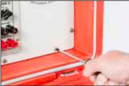
To replace the battery, remove the screws which hold the communicator panel into the top of the KMACS 5 box. Do not remove the screws which secure the communicator to the larger panel.
