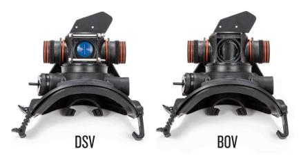
**NOTE:** The Auto Water Purge Valve Body **must be installed** if using the rebreather POD **without the regulator** (DSV) and it must be **removed if mounting the regulator to the Rebreather POD** (BOV).
