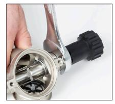
19. Tighten the Packing Nut at the Flex Knob with a <sup>15</sup>/<sub>16</sub>" wrench to the torque specifications from the correct Table (by model), see "Torque Specs" on page TORQ-1. Turn in the Flex Knob until an audible click is heard then out three full turns. This is typically very close to the optimum position to check the adjustment.
