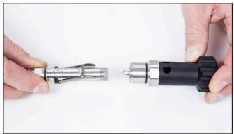
7. Unscrew the Flex Knob Assembly from the Main Tube.
