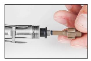
12. While holding the Inlet Valve in position, pinch each arm of the Lever Arm and slowly remove the Balance Spacer with O-ring. The Inlet Valve should remain in place. If it comes out, repeat the process until the Inlet Valve stays in place.
