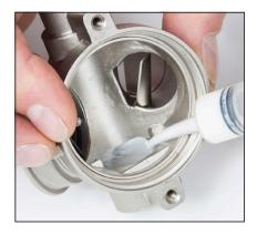
17. Lubricate the internal area of the regulator with approved lubricant where the Main Tube O-ring will insert. This is important to help prevent this O-ring from possibly getting cut when it is installed.
