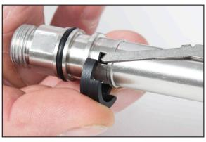
15. Install the Bearing Clip onto the outside of the Main Tube. Note that there is a locating pin on the clip that must engage the correct hole on the Main Tube. There are also small recesses on either side that the legs of the Lever Arm fit into. The clip is correctly positioned when it is in the position shown..
