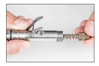
14. Lightly lubricate the ends of the Transfer Pin and install into the end of the Balance Spacer. Thread the Flex Knob Assembly onto the end of the Main Tube (closest to the lever arms) until it just stops. Hand tighten the Flex Knob Assembly and then back the Flex Knob out three turns.
