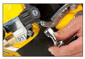
1) Disconnect the bent tube assembly at the side block end only. Loosen the jam nut at the regulator. If the bent tube will not swivel freely, you must loosen the large nut at the regulator.
