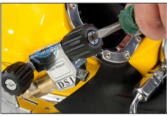
2) Remove the steady flow knob, locknut, and spring.
