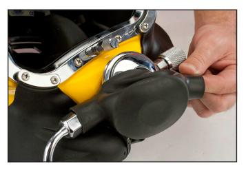
5) To install the rubber regulator cover, slide it over the bent tube assembly and stretch it over the regulator adjustment knob.
