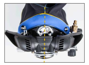
Using a torque screwdriver with a large Phillips attachment, torque the band screws to 26 inch pounds\* (2.94 Newton Meters).
