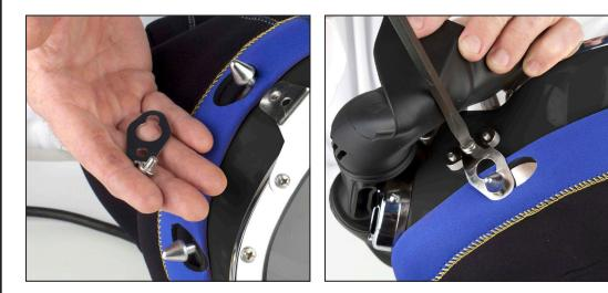
1. Remove the band keepers P/N 540-175 and 540-179.
