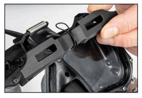
4) Bring the bracket to the top leading edge of the mask and align the holes on the bracket with the Mount Tabs on the mask.
