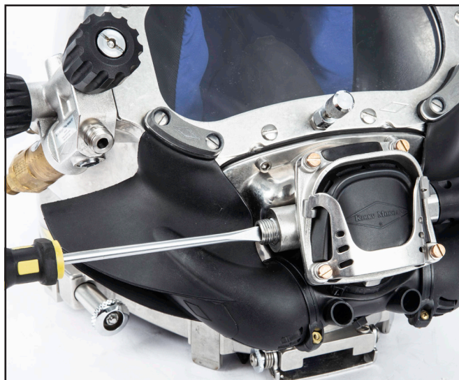
Turn the adjustment nipple 1/6 of a turn at a time to adjust the performance of the regulator.
