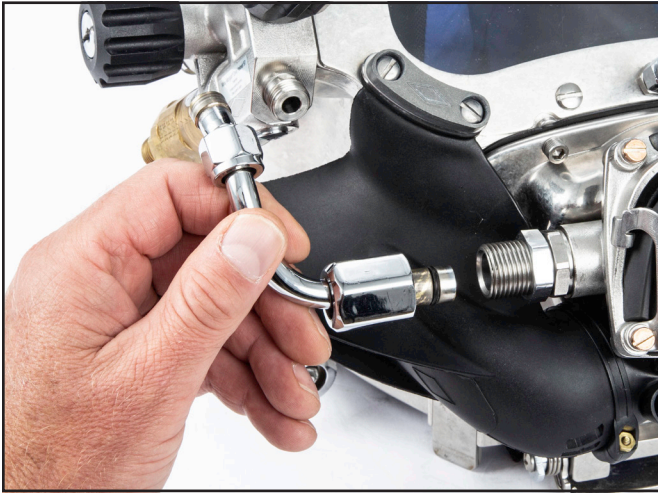
Install the bent tube assembly.
