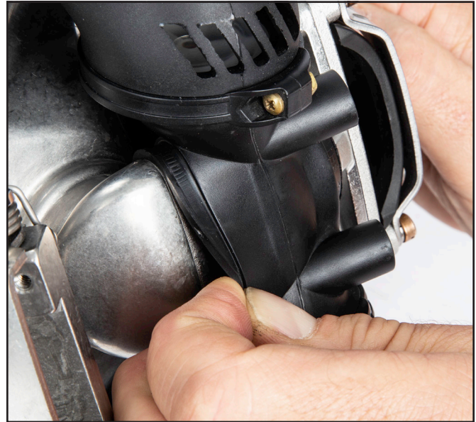
Insert the tube on the exhaust main body onto the tube of the helmet pod.
