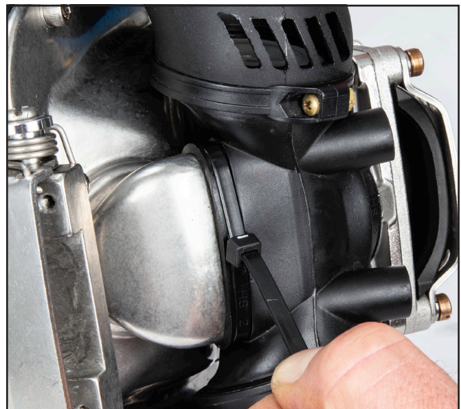
Secure and seal with a tie wrap.
