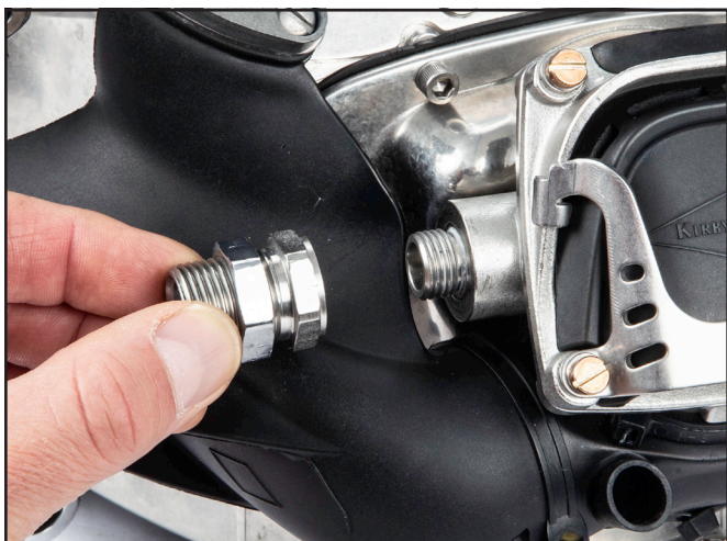
Remove the bent tube adapter.
