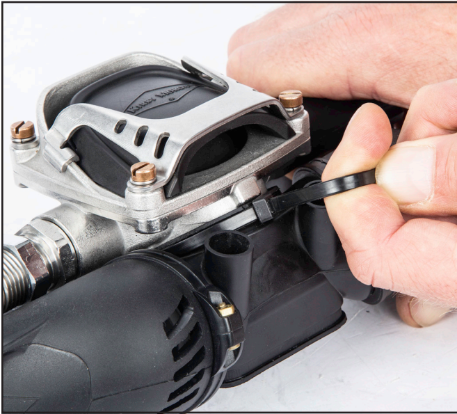
Install the tie wrap on the regulator.
