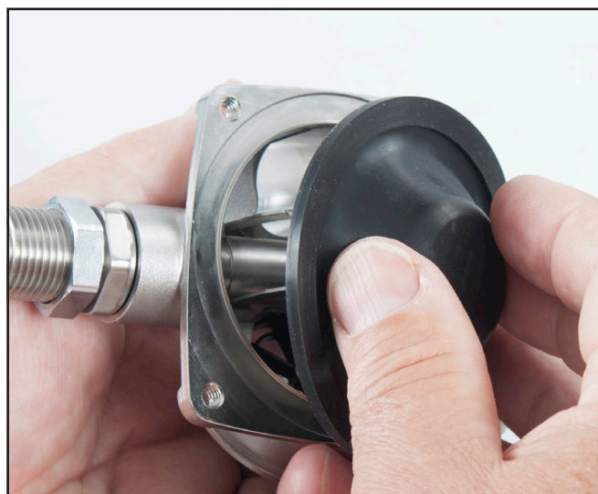
Place the diaphragm onto the regulator body.
