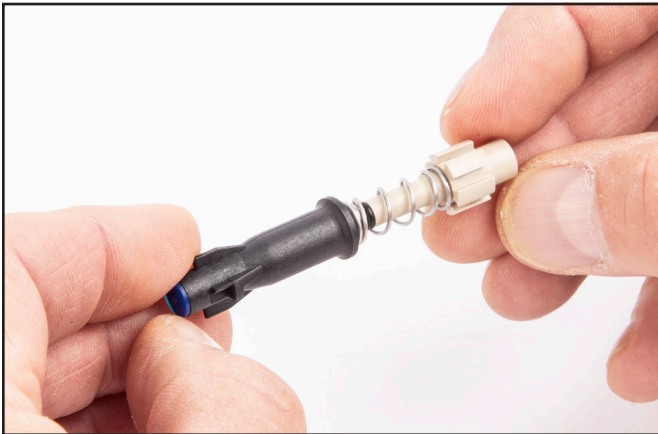
Using the balance spacer with the O-ring installed, insert the O-ring into the open end of the inlet valve and stop.
