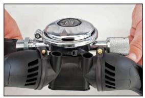
2. Place the tie wrap P/N 520-042 around the tie wrap seating surface on the exhaust assembly and tighten. Make sure that the tie wrap end is positioned as shown. Cut off the excess tie wrap tail.
