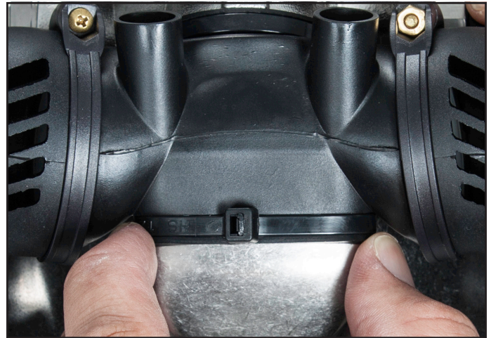
The Quad Valve must be properly connected to the regulator and the water dump cover on the pod.
