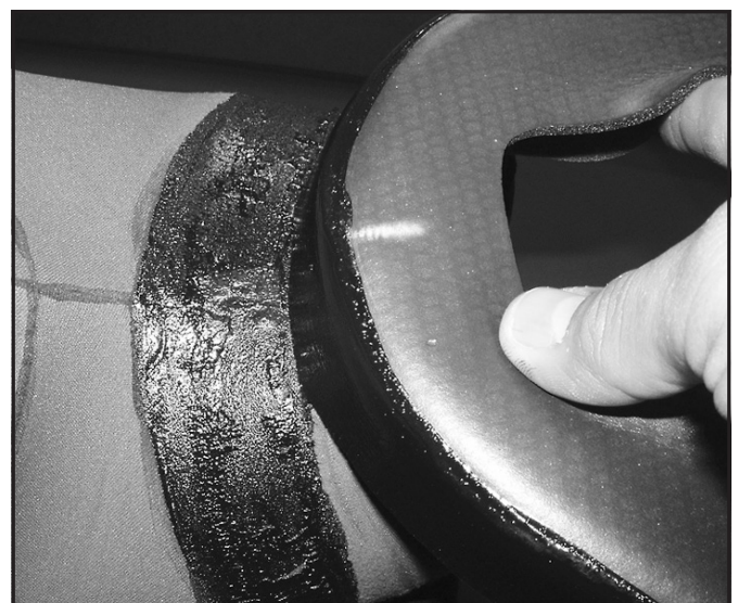
The foam side of the face seal must be oriented correctly in relationship to the hood.
