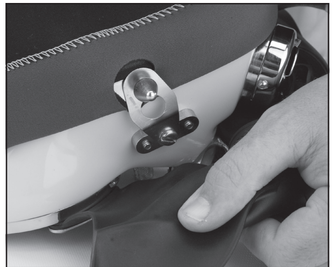
To access the bottom band keeper, the exhaust whisker must be moved out of the way then tighten the bottom band keeper.
