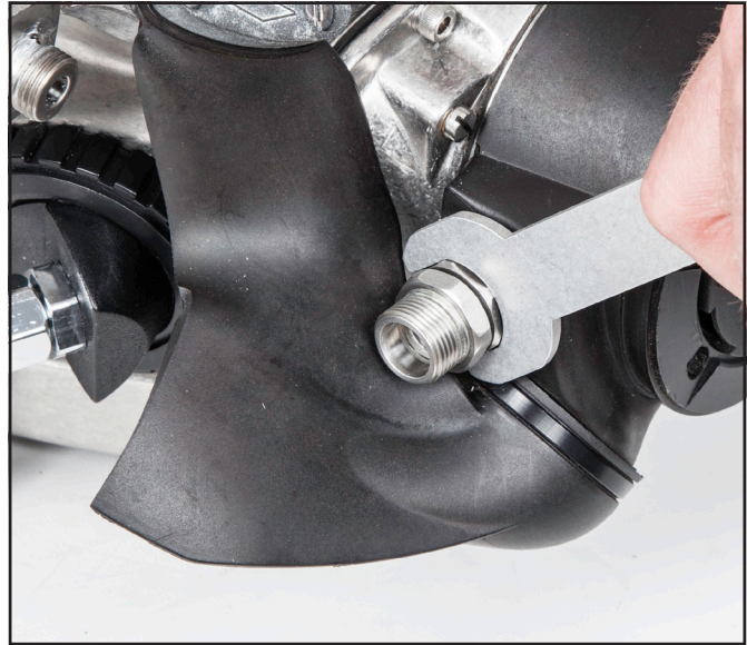
Ensure that the adjustment lock nut is tight against the REX® regulator body
