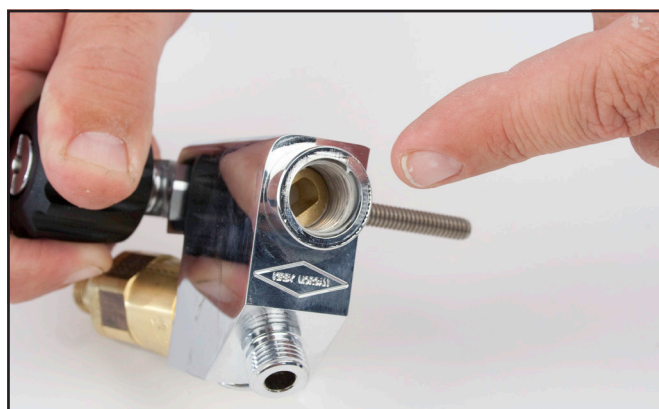
The seat should be removed for inspection.
