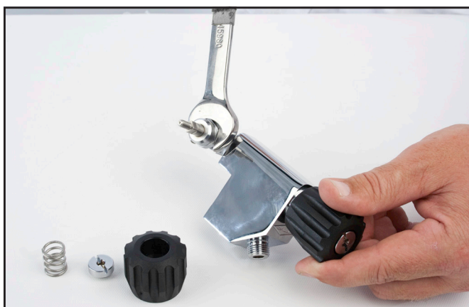
Undo the packing nut.
