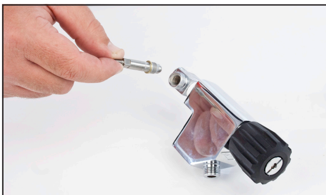
Remove the valve stem.
