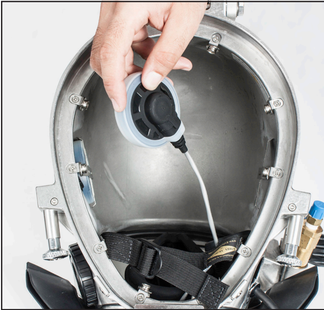
Remove the earphones from the earphone retainers.
