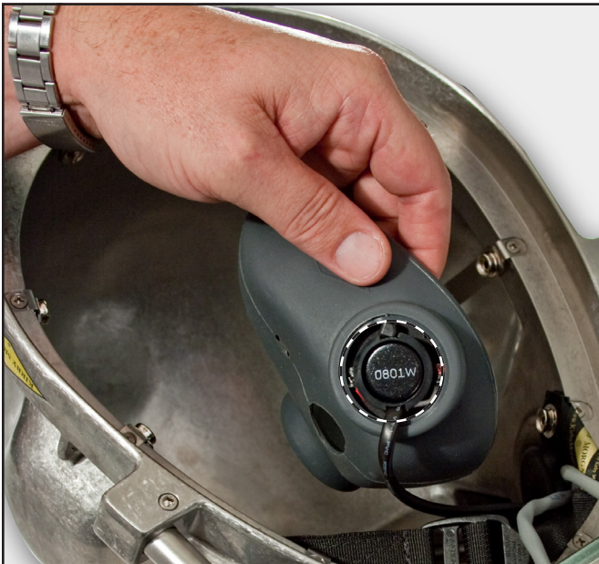
The microphone must be removed from the oral nasal mask.
