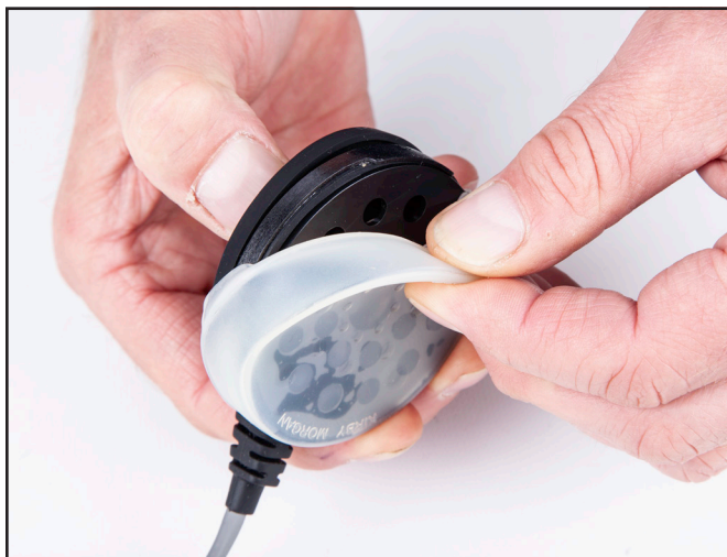
Removing the rubber cover from the earphone.
