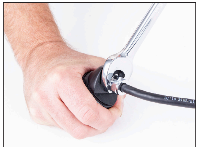
Use a 3/4 inch wrench to unscrew the waterproof connector.
