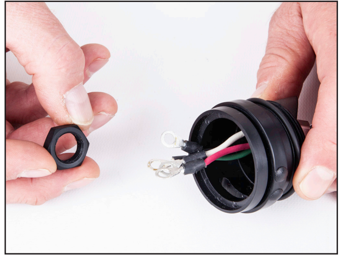
3. Using a 3/4 inch wrench, tighten the waterproof connector.
