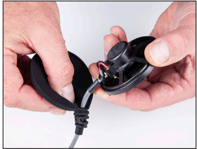
Inspect the mylar earphone.
