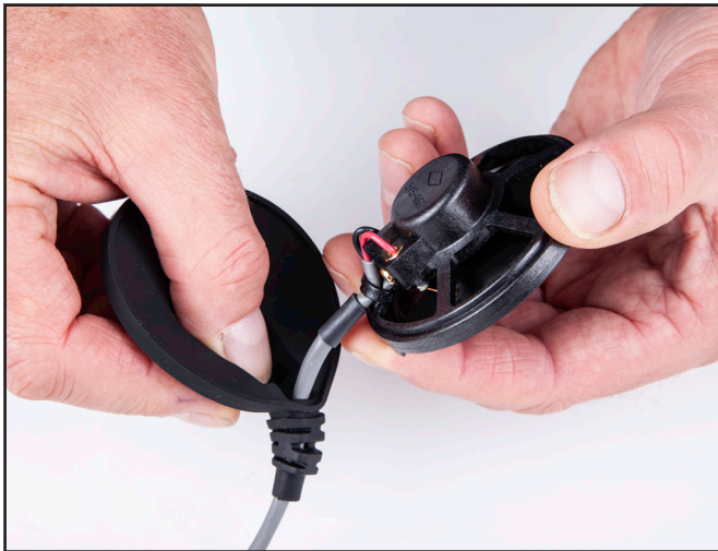
3. Cut the tie wrap that secures the wire assembly to earphone.
