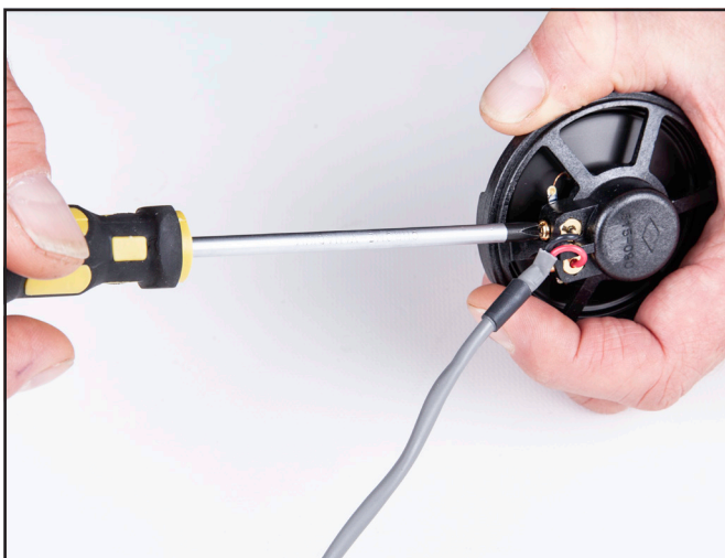
5. Pull both black and red wires out and away from Earphone Speaker.
