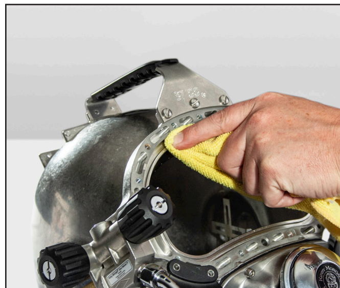
Clean the O-ring groove prior to replacing the face port O-ring.
