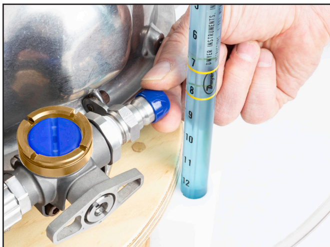
9. Ensure SBV is in open position (parallel).
