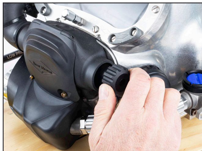
13. Ensure the EGS and Steady Flow valves are closed BEFORE the EGS supply tank is turned on.
