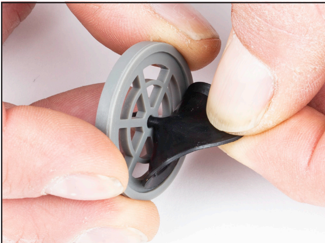
8. Remove old valve from Valve Seat Insert.
