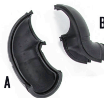
HOT WATER TUBES
