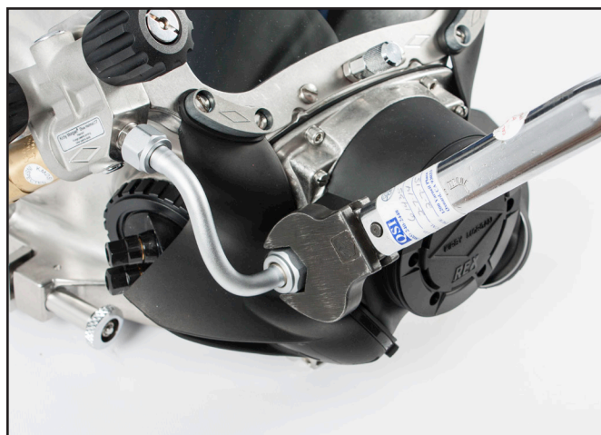
Make sure the connection between the bent tube and the regulator is snug.
