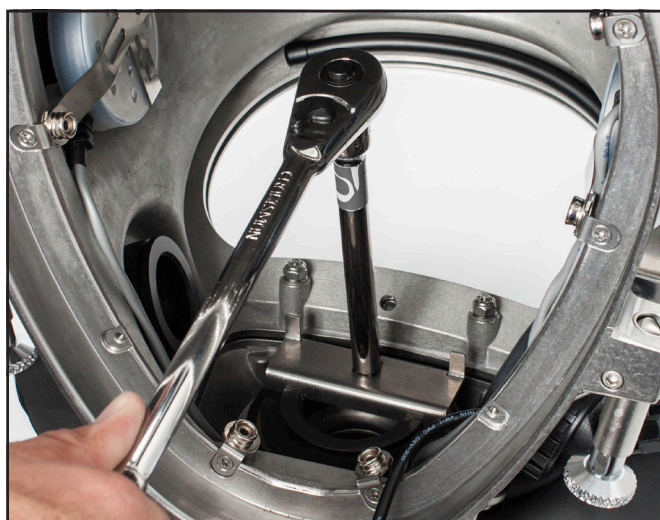
The regulator mount nut must be tightened. See "Torque Specs" module. Use a torque wrench to ensure the correct setting.
