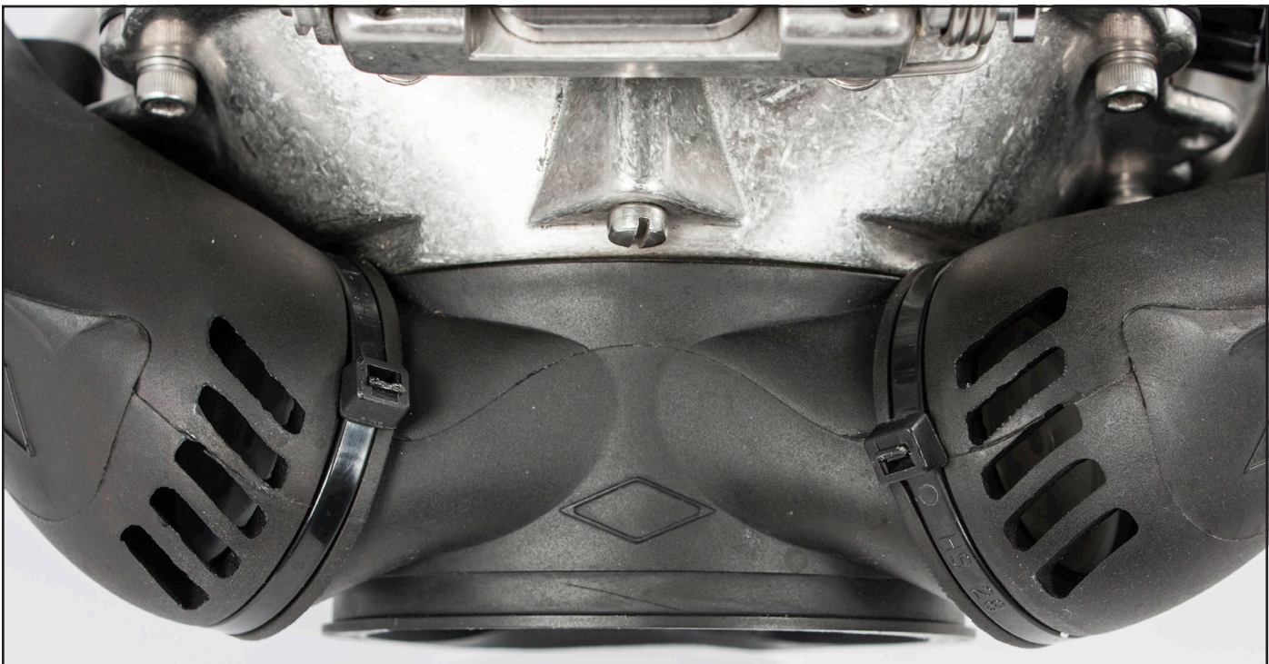
The port and starboard whiskers should align so that the parting line on the bottoms of the wings is lined up with the parting line on the main body, and the heads of the tie wraps are positioned on the back of the body. You can also make marks on the whiskers with a felt tip pen.
