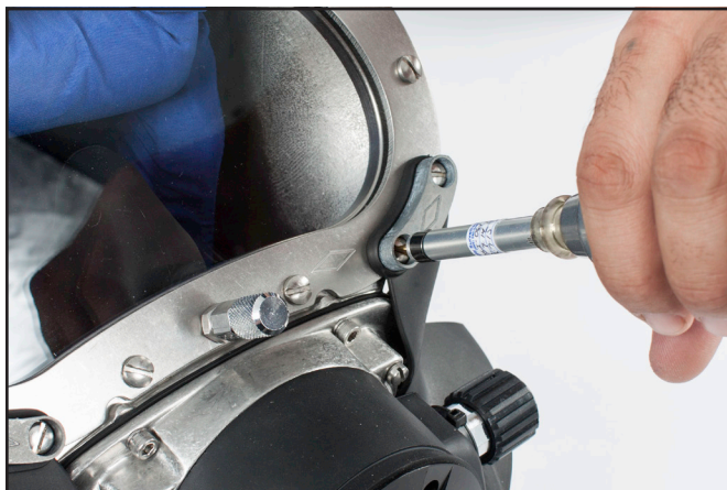
Only use a torque screwdriver to tighten the screws that secure the whiskers to the face port.
