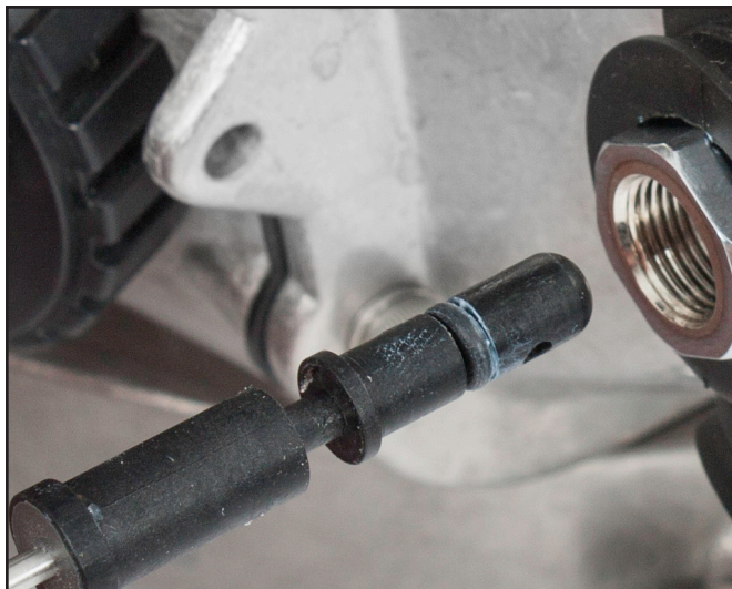
If you install a new seat on the inlet valve, you must allow the silicone sealant time to dry. Be sure the O-ring is properly installed on the valve body.
