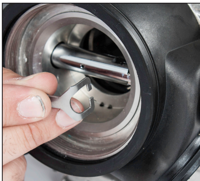
The roller lever is installed after the horseshoe is installed.
