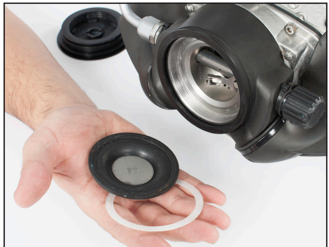
Remove the diaphragm and washer.
