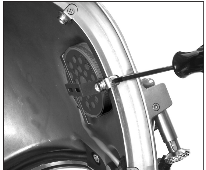
Removing the snap tab that also holds the earphone retainer.
