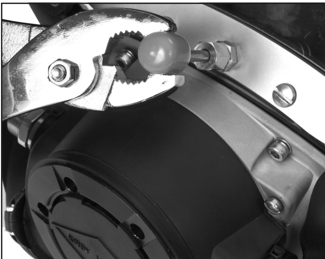
Protect the nose block device knob with a plastic cap or rag when you remove it.
