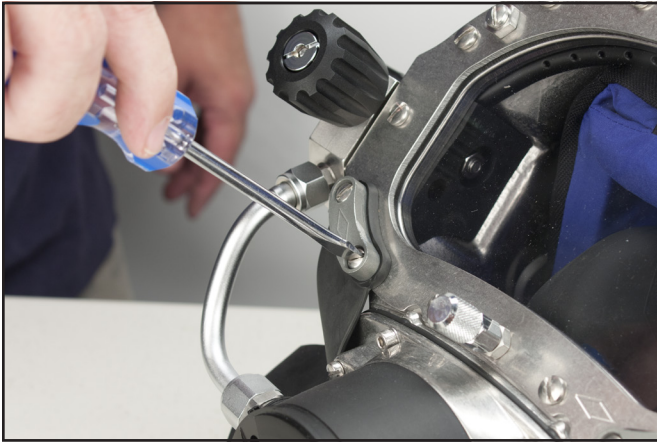
Remove the screws that secure the zinc anodes, whisker spacers and whiskers.
