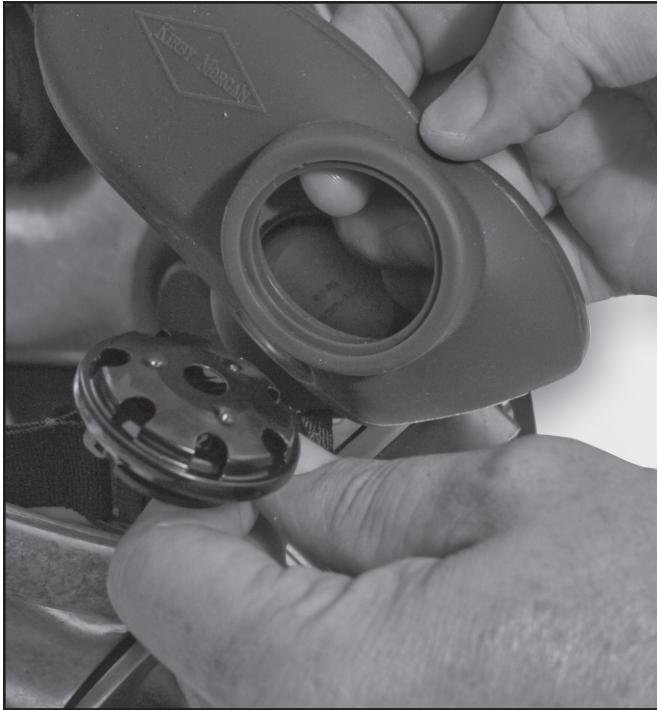
Remove the nose block device, microphone, and oral nasal mask.
