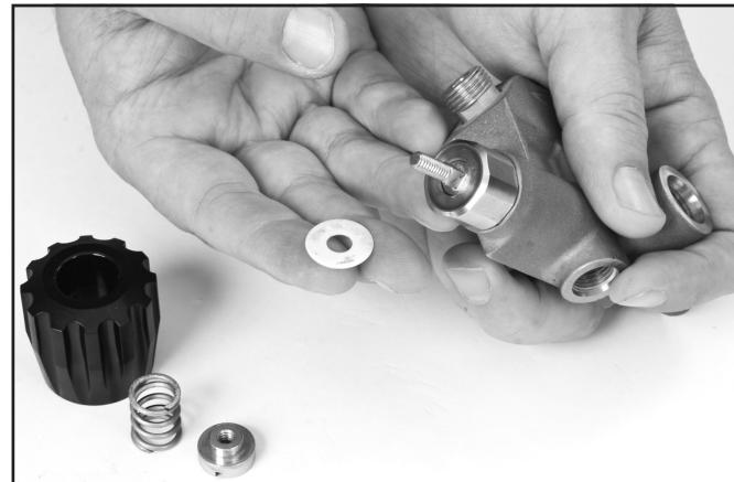
*Do not lose the washer that sits between the defogger valve knob and the bonnet.*
