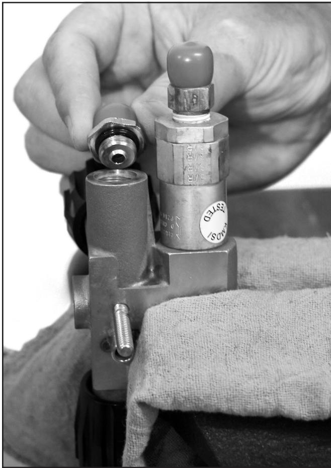
The adapter or inlet nipple for the EGS valve should be removed periodically to inspect the O-ring and to make cleaning of the side block interior easier. Note that the stud which is used to mount the side block is fastened with Loctite® 222. This is a dealer serviceable item only.
