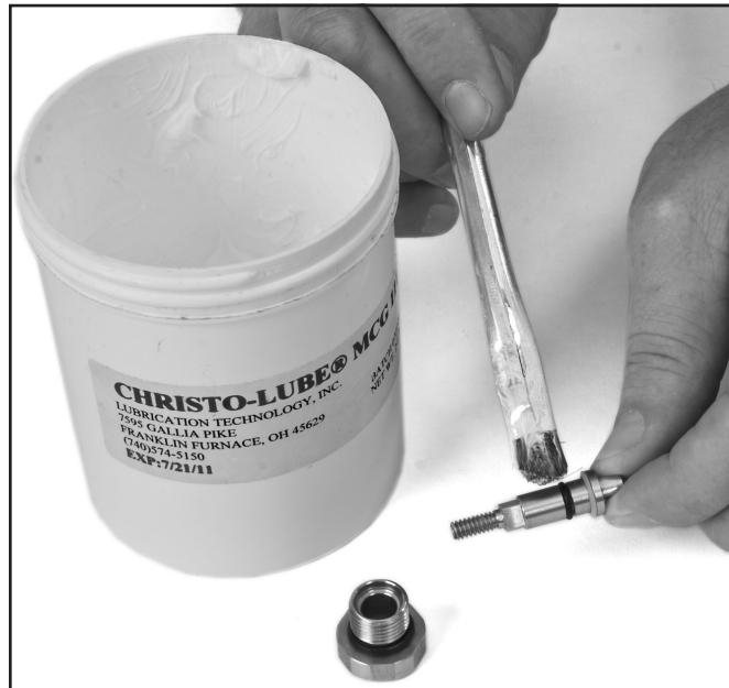
*All internal moving parts (with the exception of the valve seat) and O-rings should be regularly lubricated.*
