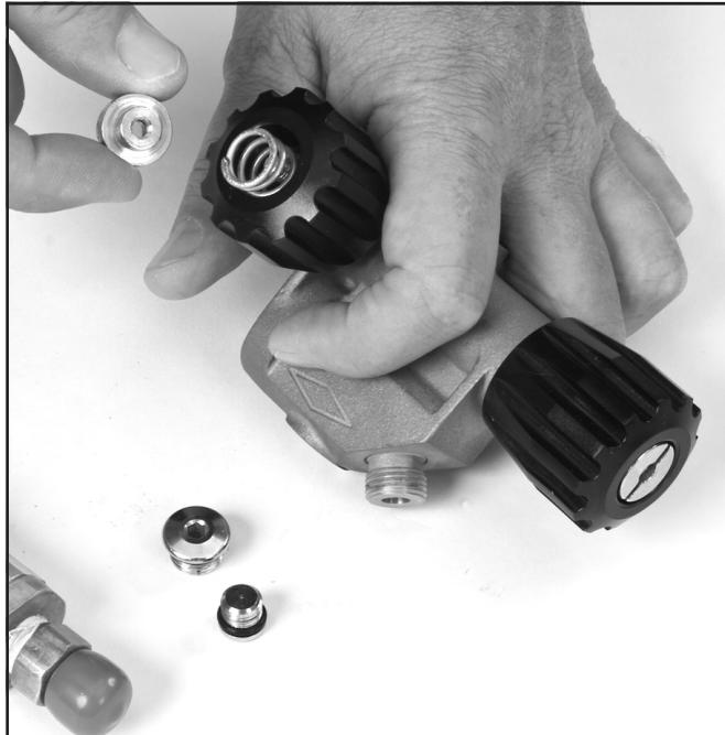
*Remove the lock nut and spring*
