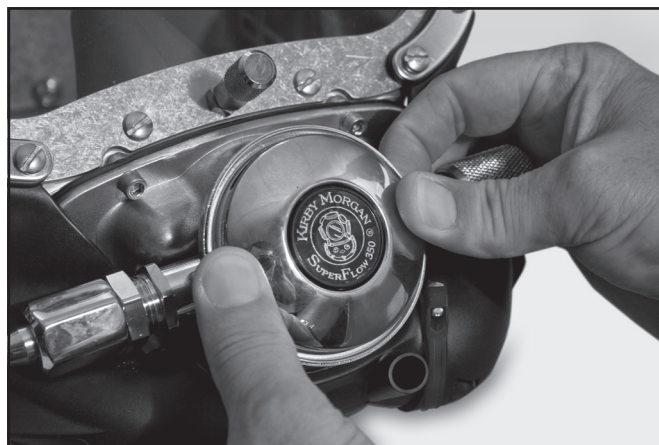
Press the cover over the diaphragm.
