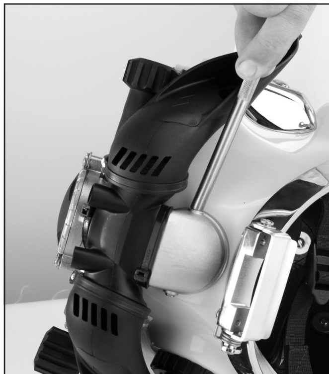
Tighten the screws that connect the quad exhaust cover to the exhaust body.
