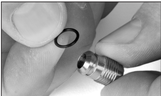
Install the O-ring on the inlet nipple.
