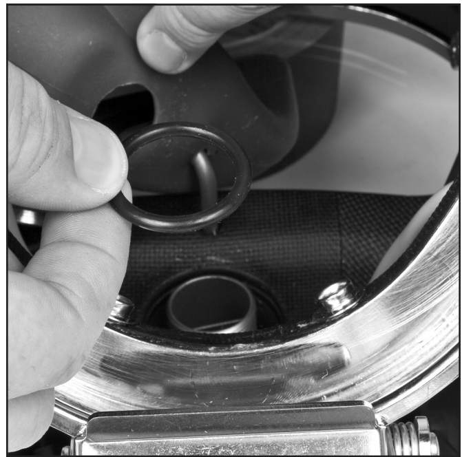
Install the O-ring that mounts on the regulator tube inside the helmet.
