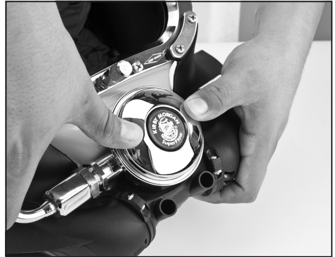
Push down on the regulator cover to simulate a tightened clamp.
