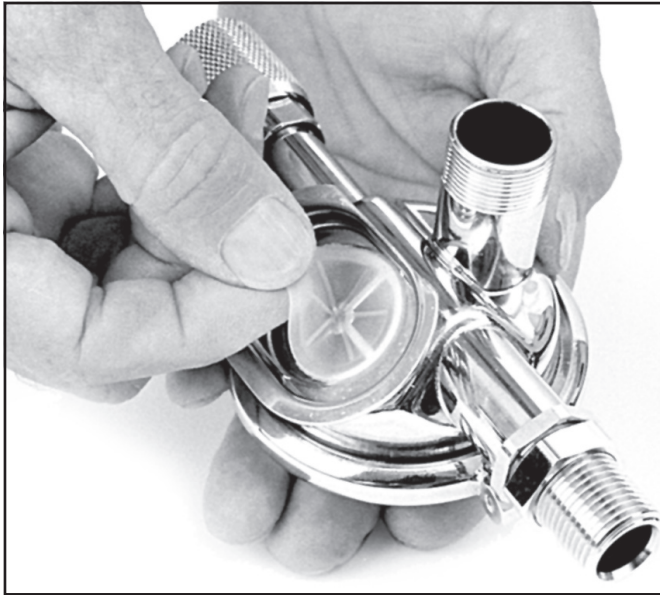
The exhaust valve must be in good condition if you intend to reuse it.
