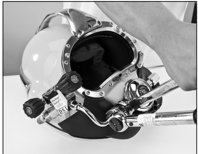
The jam nut and bent tube must be tightened to the proper torque specification.
