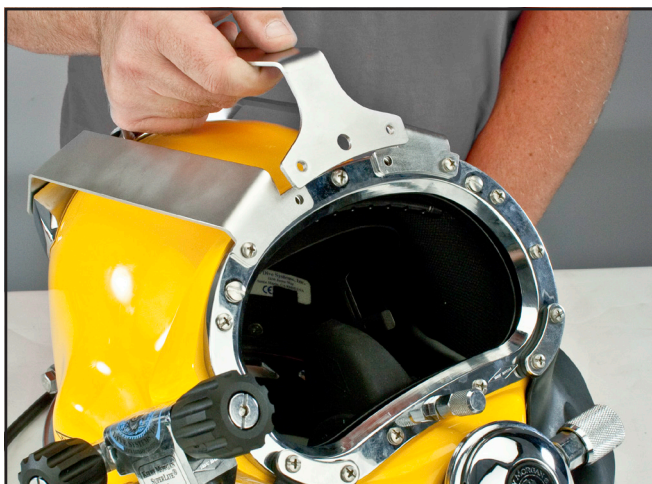
Position the handle on the helmet.
