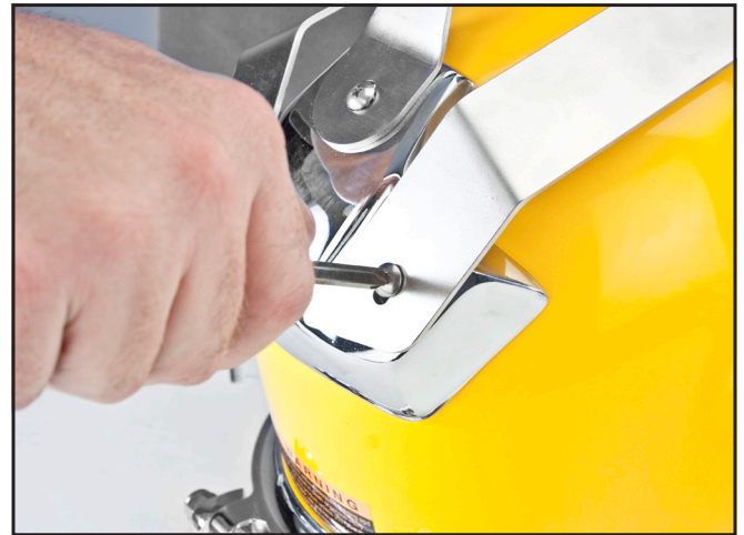
Remove the screw at the rear of the handle.
