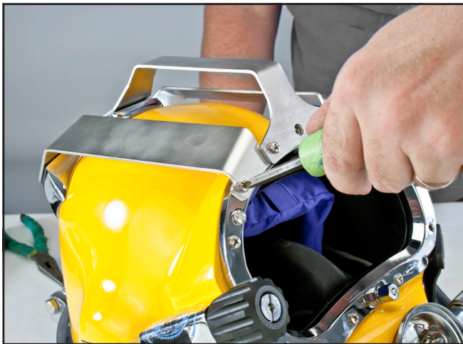
Remove the front mount screws
