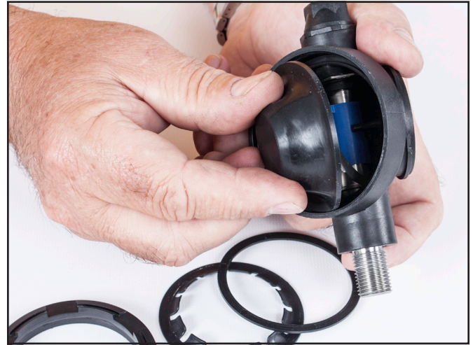
Remove the diaphragm.
