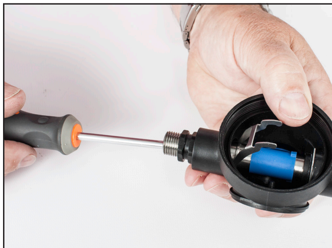
Using a medium flat blade screwdriver, rotate the adjustable nipple inward, (clockwise) slowly while observing the lever arm for ANY slight movement.
