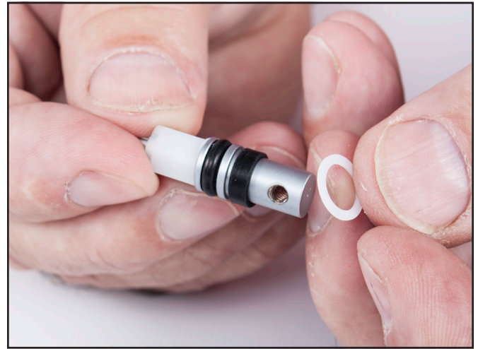
Install the spacer and thrust washer onto the adjustment shaft.
