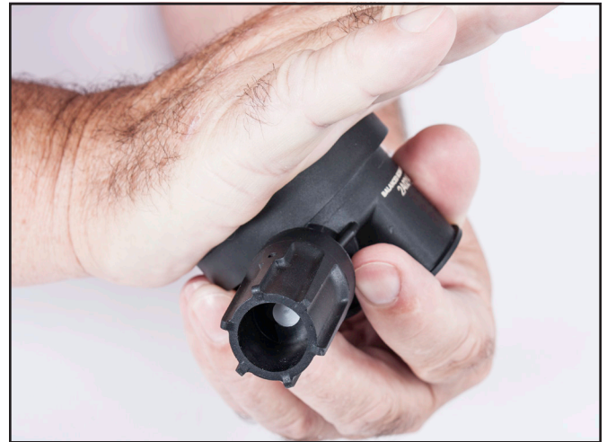
Tighten the diaphragm retainer ring with the palm of the hand until this ring and the regulator housing top surface make contact.
