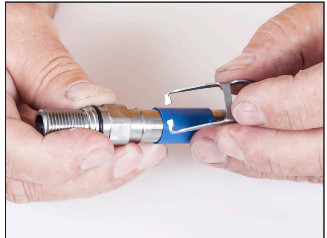
Remove the lever arm.
