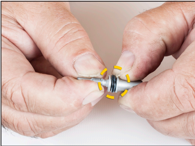
Remove the O-ring.
