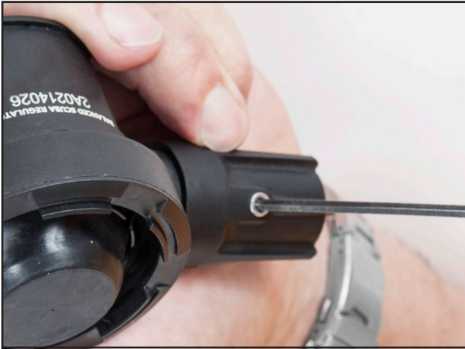
Remove the adjustment knob screw.
