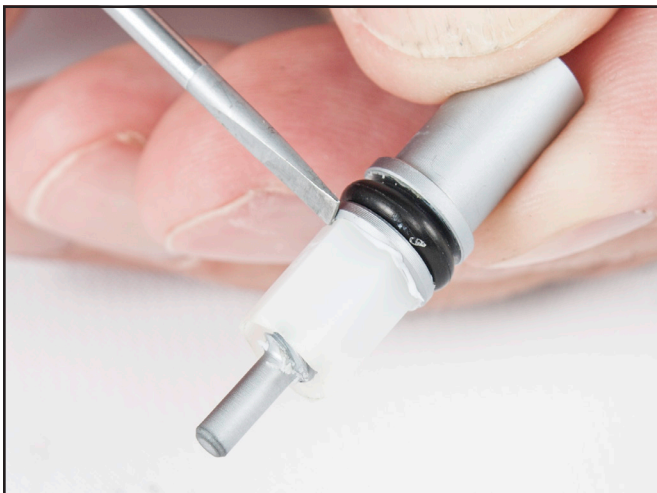
Install the spring seat, FLAT END onto the threads of the adjustment shaft and thread it on all the way until it stops.
