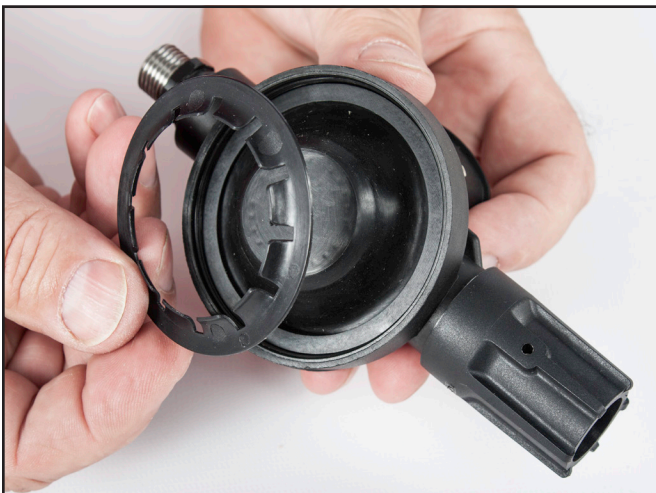
Install diaphragm surge dam.
