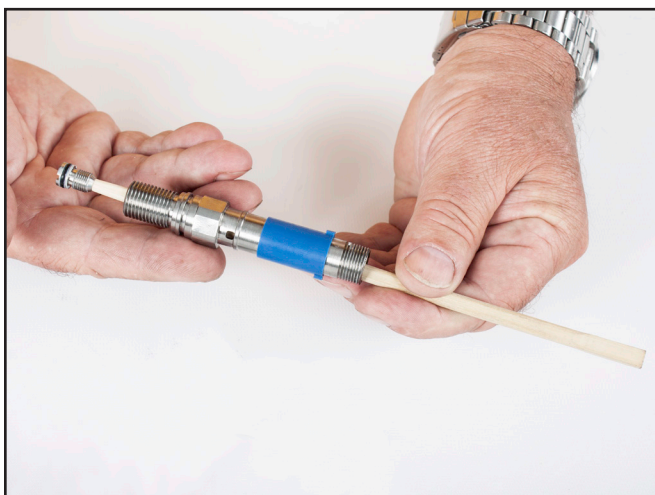
Push the adjustable nipple out with a wooden dowel or chop stick to prevent damage to the sealing edge of the nipple
