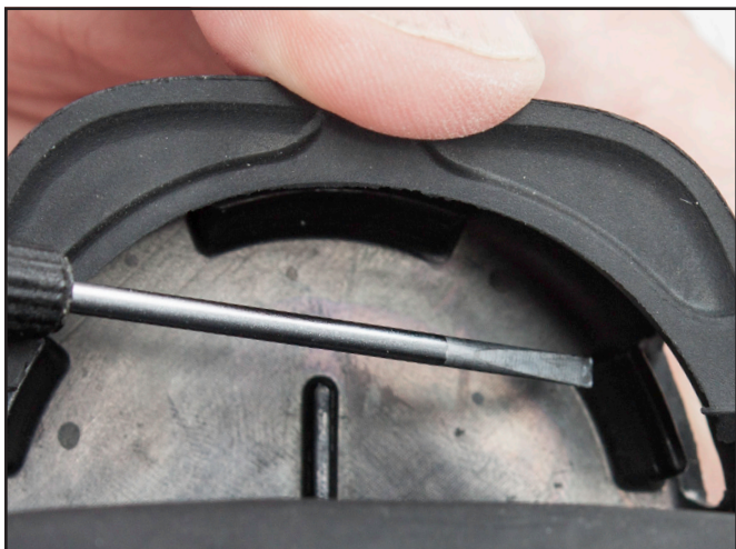
Notice the important standoff features of the inside of the regulator shroud/exhaust cover.
