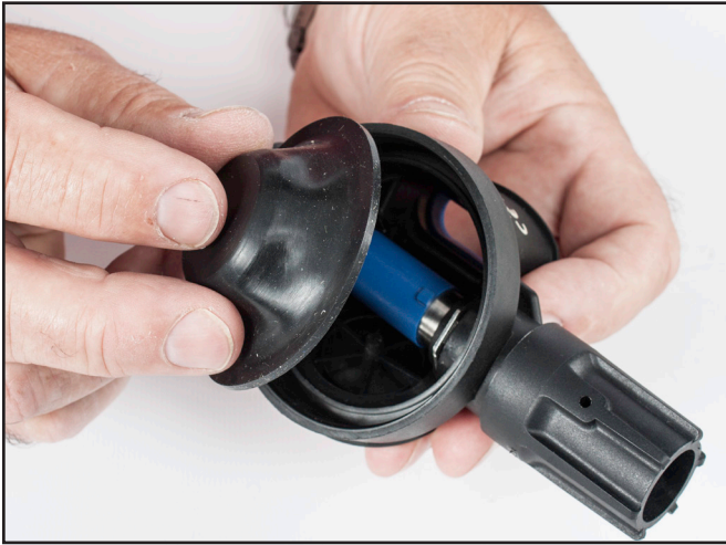
Install the diaphragm.
