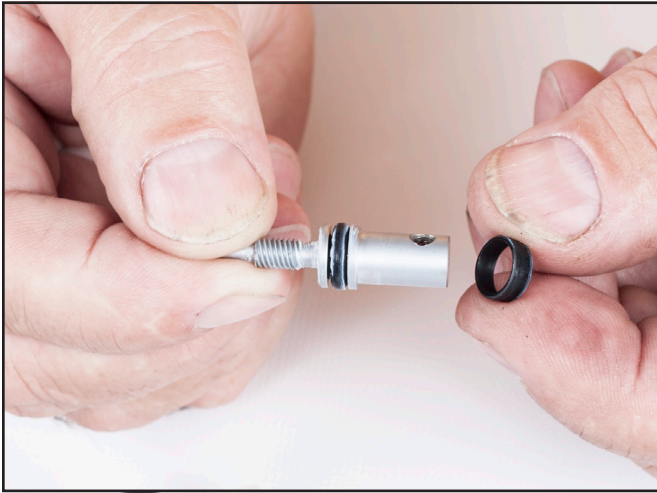
Separate the spacer.
