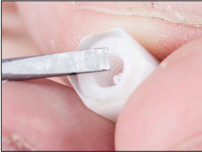
Look closely at the spring seat one end is recessed (shown above) and the other is flat.
