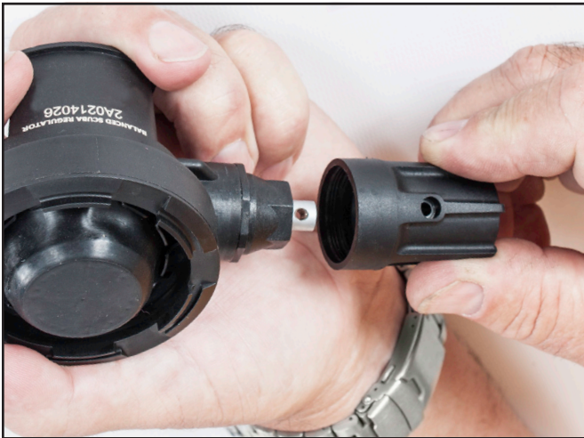
Remove the adjustment knob.
