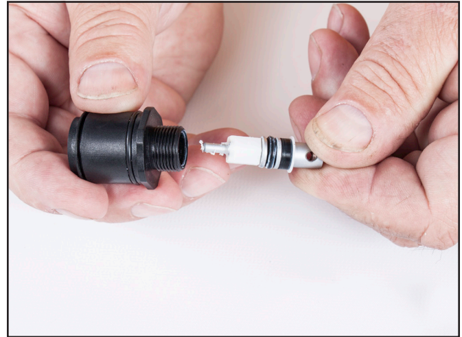
Remove the adjustment shaft.
