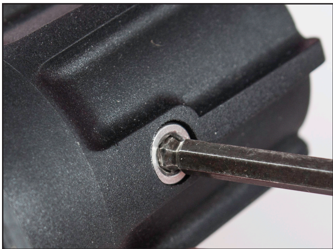
Tighten until the top of the hex end is just barely below the outer surface of the adjustment knob.
