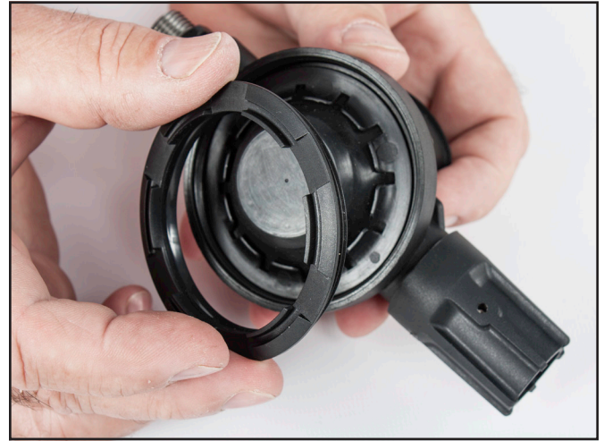
Install diaphragm retainer ring.
