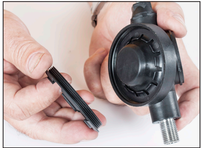
Using the palm of your hand loosen and remove the diaphragm retainer ring.
