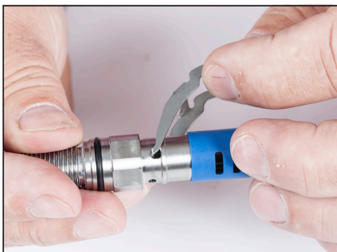
Note the orientation of the lever arm to the main tube.
