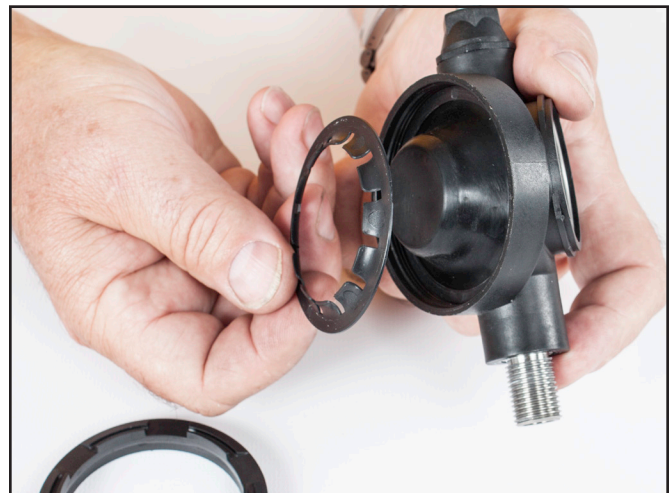
Remove the surge dam.
