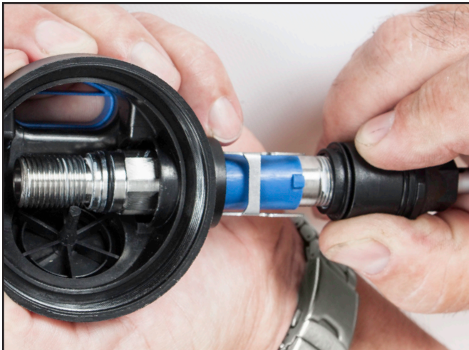
Push on the threaded hose end of the main tube while depressing the lever arm then pull it straight out from the regulator housing.
