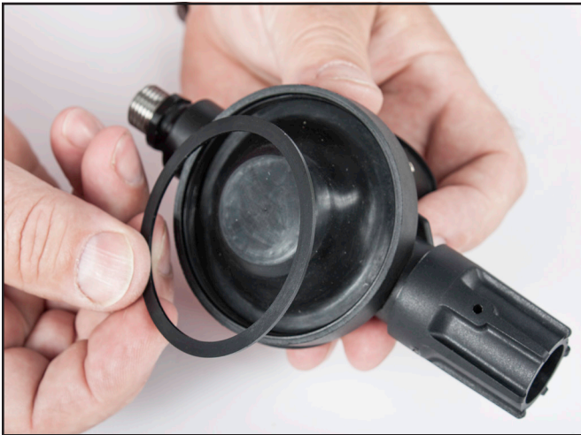
Install the diaphragm washer.
