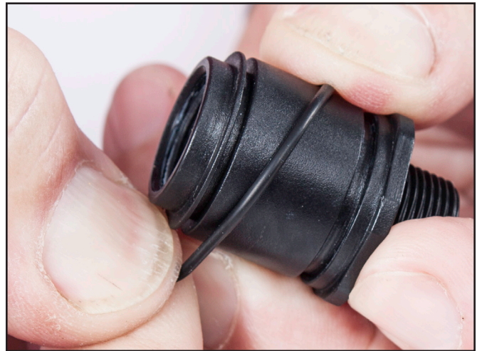
Lubricate O-ring and install onto the adjustment guide insert.
