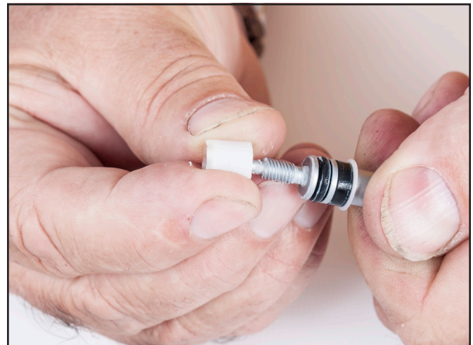
Separate the spring seat.
