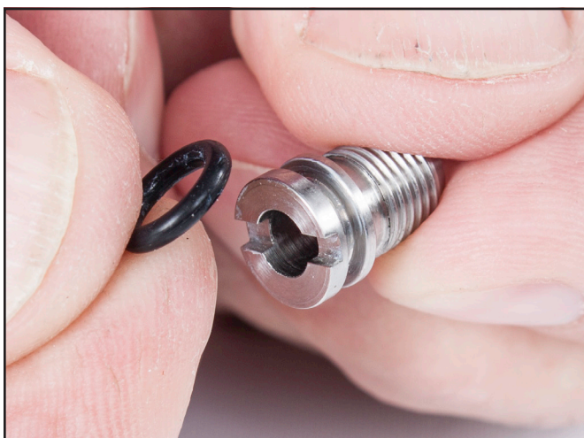
VERY lightly lubricate the O-ring and install onto the adjustable nipple.
