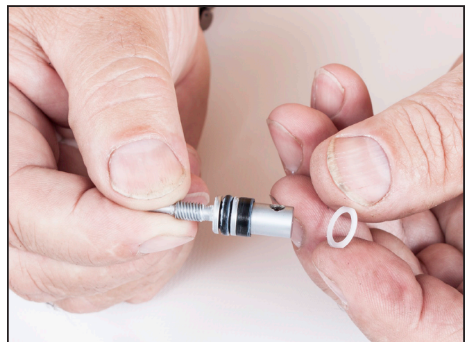
Separate the thrust washer.
