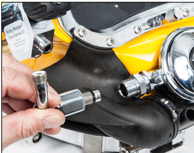
Removing the bent tube.
