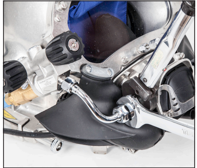
For the SuperFlow® 450 and 455 Balanced regulators, torque the jam nut against the bent tube mount nut. See "Torque Specs" module for correct torque.
