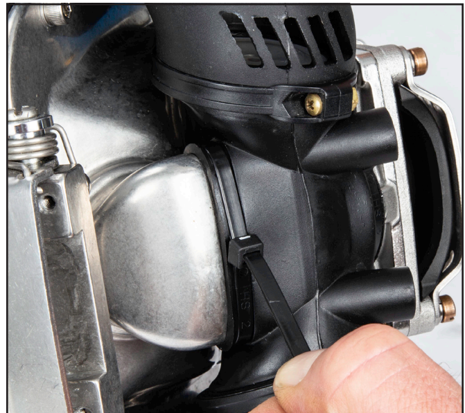
Secure and seal with a tie wrap.
