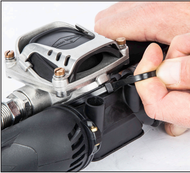
Install the tie wrap on the regulator.
