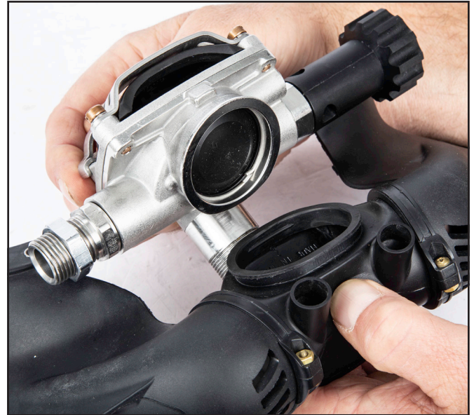
Install the main exhaust body onto the exhaust flange of the regulator body.
