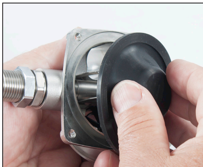
Place the diaphragm onto the regulator body.
