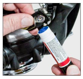
1. Apply Loctite® 248 to the screws that secure the chin strap.
