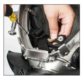
3. Tighten the screws with a torque screwdriver in accordance with the torque specification found in the correct table (correct model) of the manual. See "Torque Specs" module.
