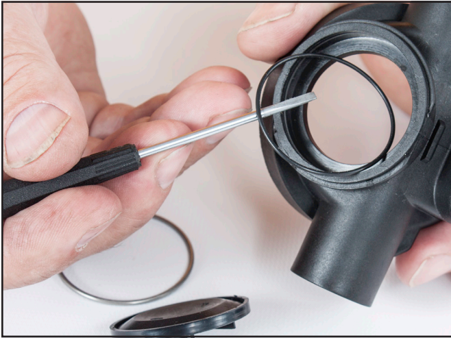
Carefully remove the O-ring for the exhaust valve insert.
