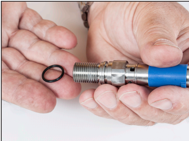
Remove the O-ring from the main tube.
