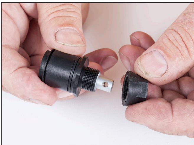
Remove the end cap packing nut.
