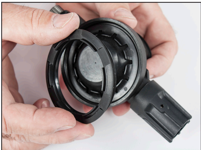
Install diaphragm retainer ring.
