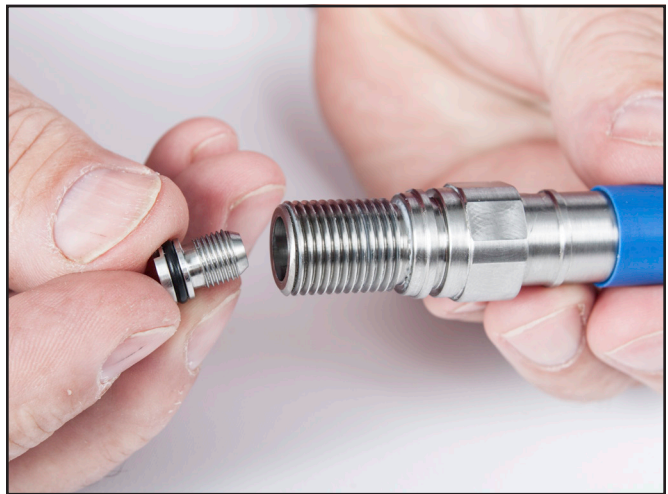
Insert the adjustable nipple subassembly into the main tube.
