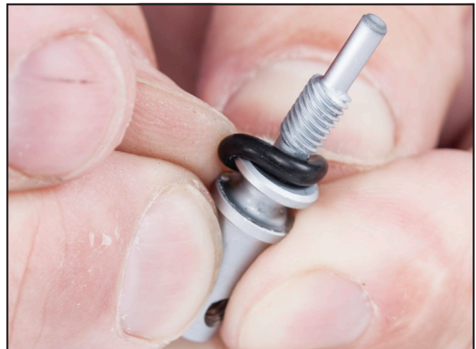
Lubricate O-ring and install onto the adjustment shaft.
