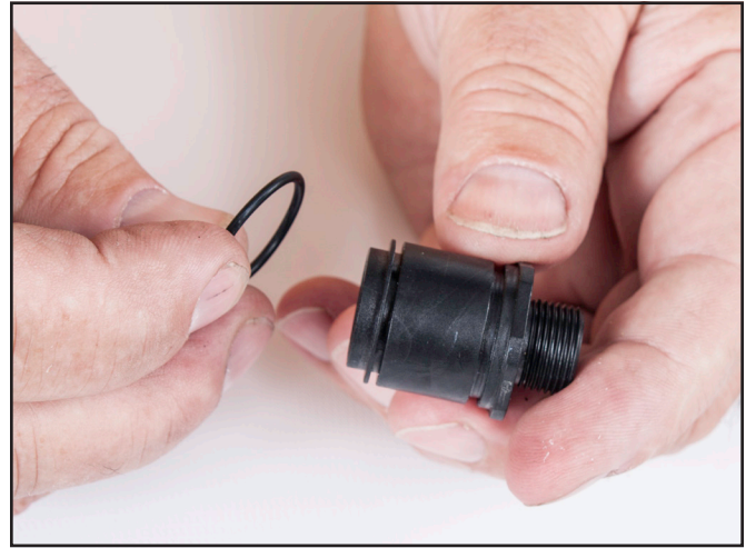
Remove the O-ring from the adjustment guide insert.
