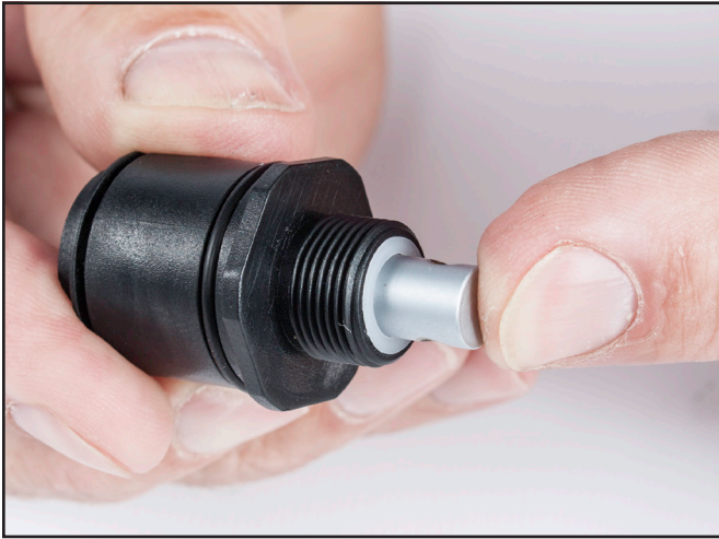
Push all of the components on the adjustment shaft into the adjustment guide insert.
