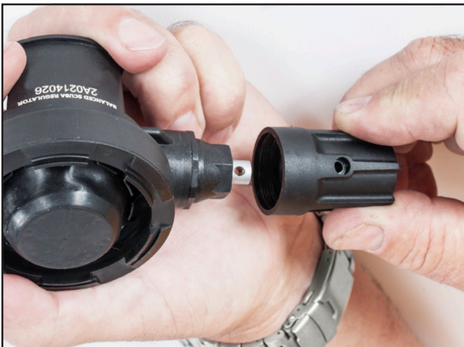
Remove the adjustment knob.
