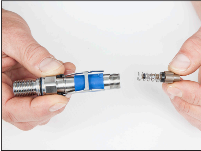
Remove the balance spacer, spring and washer.
