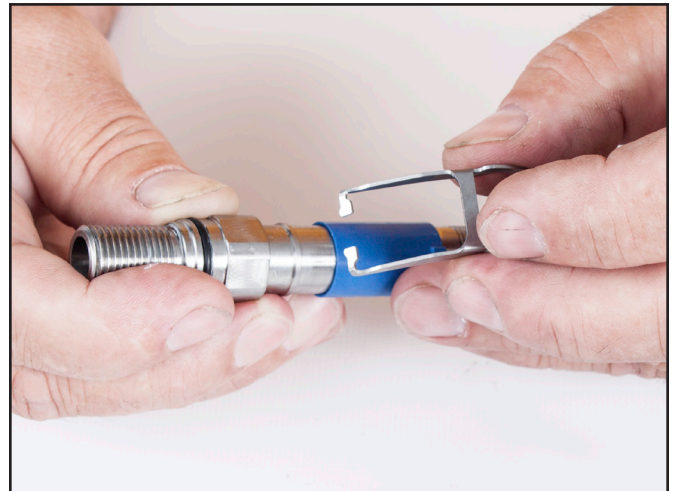
Remove the lever arm.
