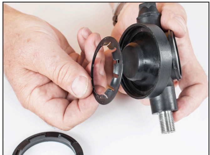
Remove the surge dam.
