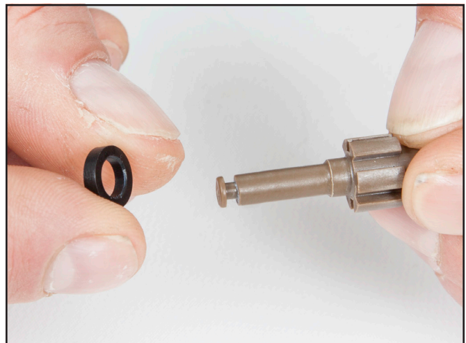
Install the washer onto the balance spacer
