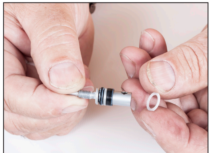
Separate the thrust washer.
