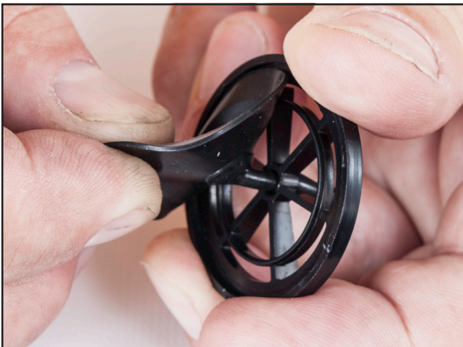
Separate the exhaust valve insert and exhaust valve.
