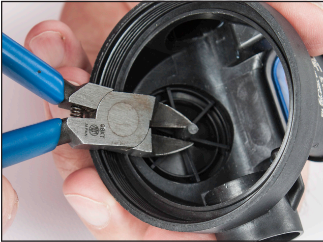
Install the exhaust valve and cut off excess material.
