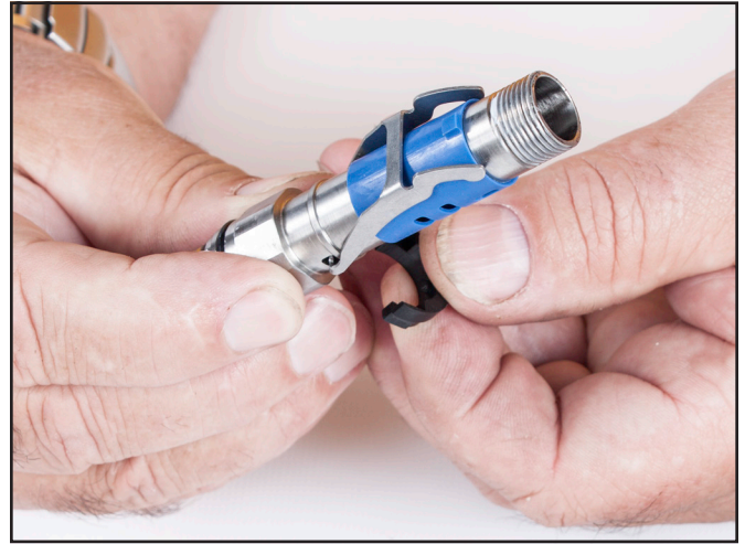
Remove the lever bearing clip from the main tube.
