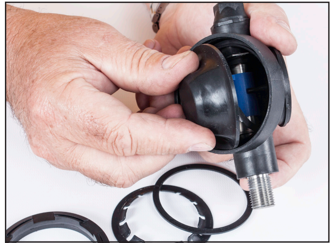
Remove the diaphragm.
