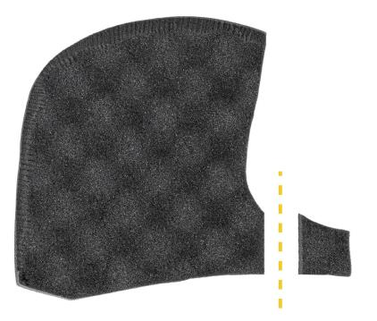
The small section on the right of both side foams is now trimmed to better accommodate the new LVON.
