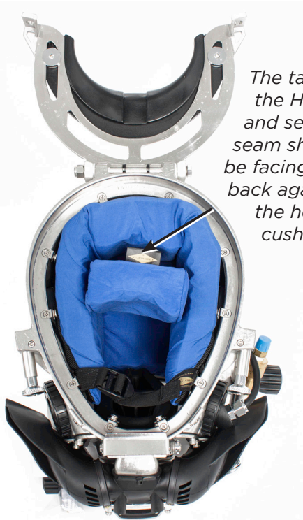
Proper installation and alignment of the HCFS in the helmet.
