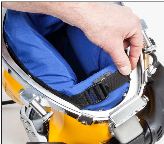
The chin strap is tightened on the outside of the chin cushion as to press the chin cushion snug against the divers chin.
