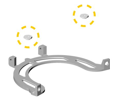
P/N 550-113 Neck Pad Adjustment Nut, circled above, is now made from stainless steel.
