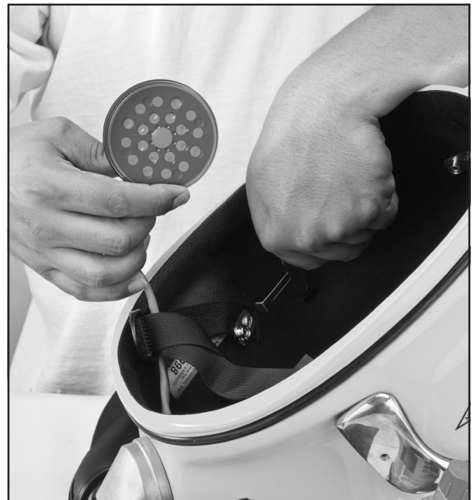
Remove the earphones from the retainers to inspect the speaker cones.
