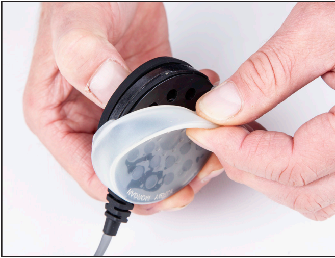
Removing the rubber cover from the earphone.
