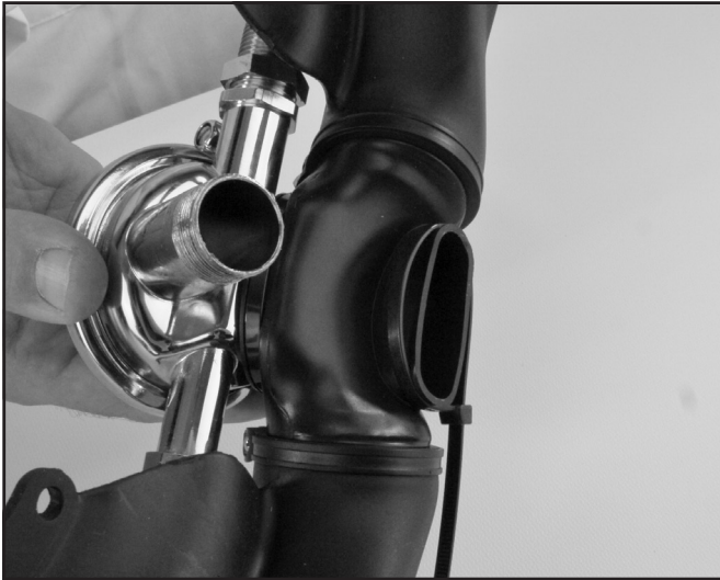
Pre-install the tie wrap.
