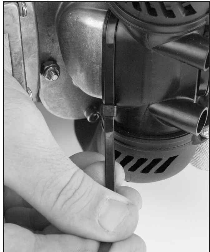
Carefully tighten tie wrap.
