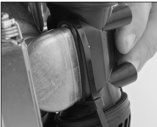
Insert the regulator into the pod.
