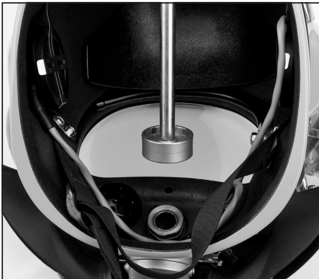
The regulator mount nut must be loosened with a wrench.
