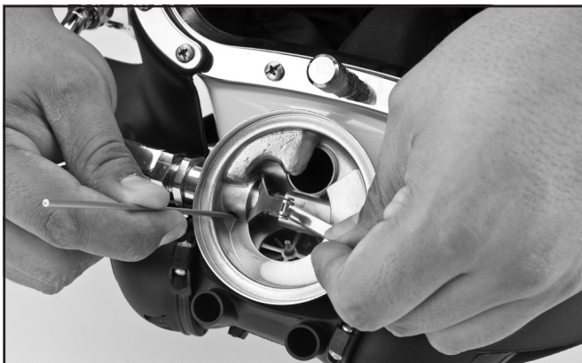
Insert the inlet valve holding tool into the balance hole on the inlet tube.
