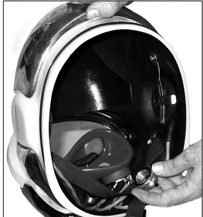
Remove the mount nut from the regulator.
