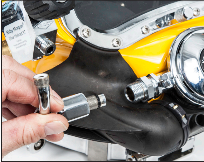
Removing the bent tube.
