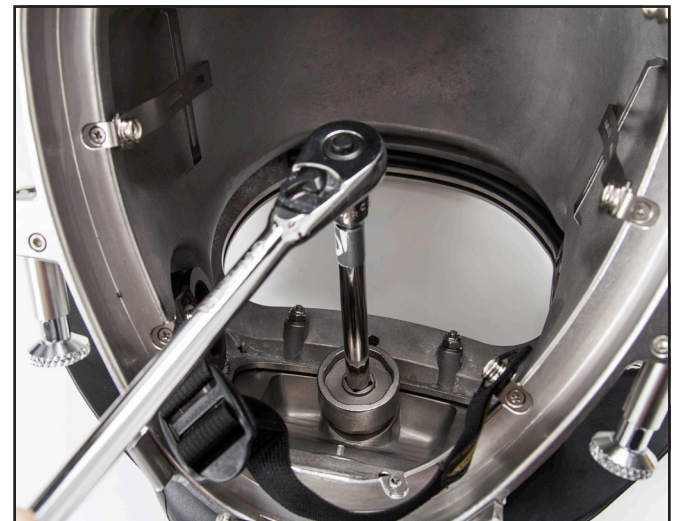
Removal of the regulator mount nut.
