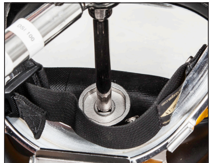
Removal of the regulator mount nut.
