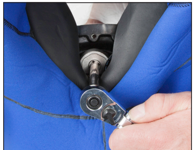
Removal of the regulator mount nut.
