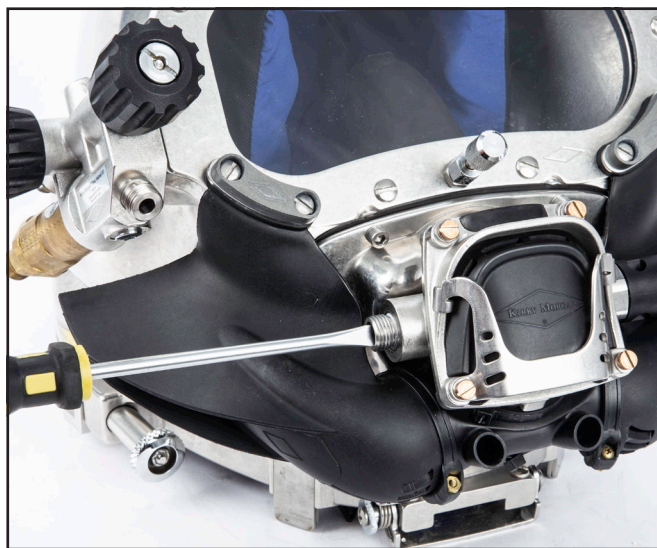
Turn the adjustment nipple \frac{1}{6} of a turn at a time to adjust the performance of the regulator.
