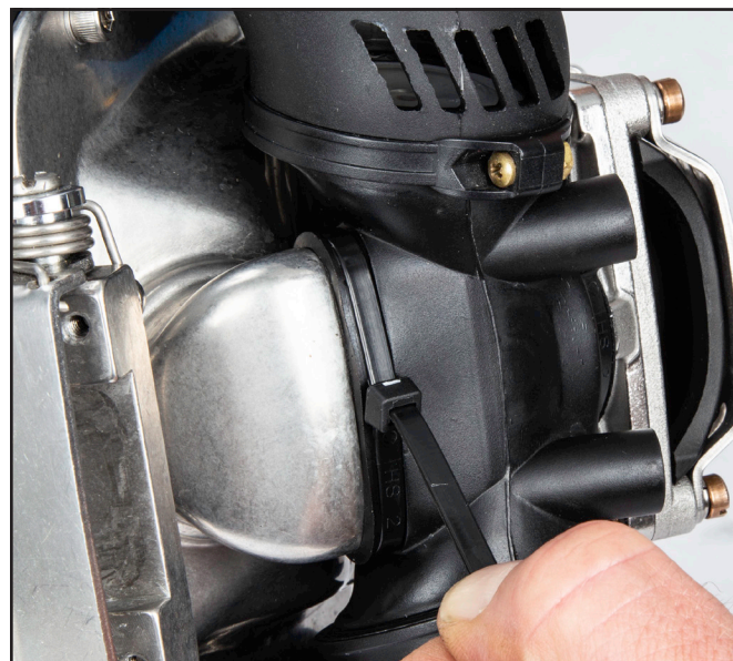
Secure and seal with a tie wrap.
