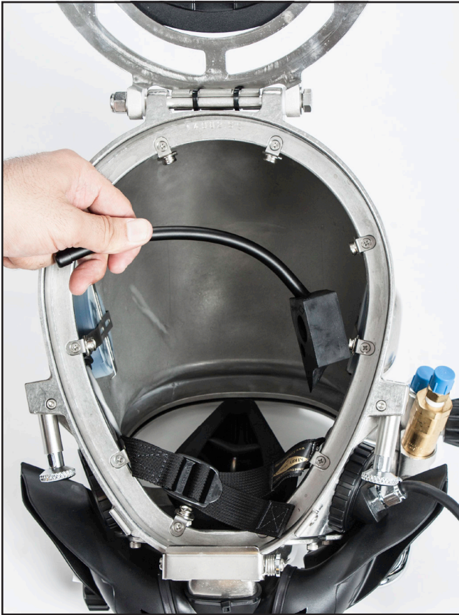
Remove the air train along with the air train body.
