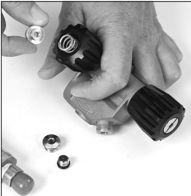
Remove the lock nut and spring
