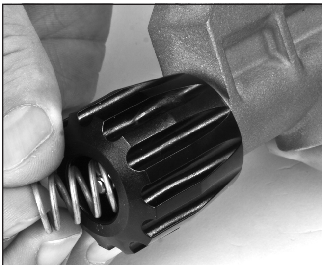
Install the spring in the steady flow valve control knob.
