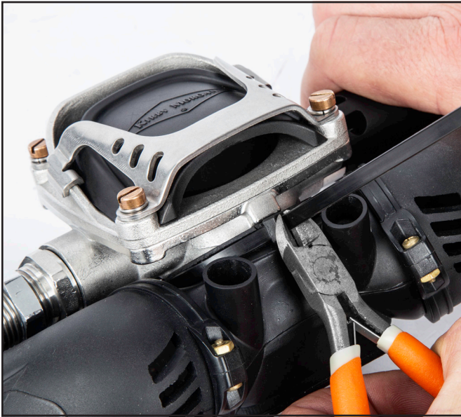
Remove excess tie wrap.
