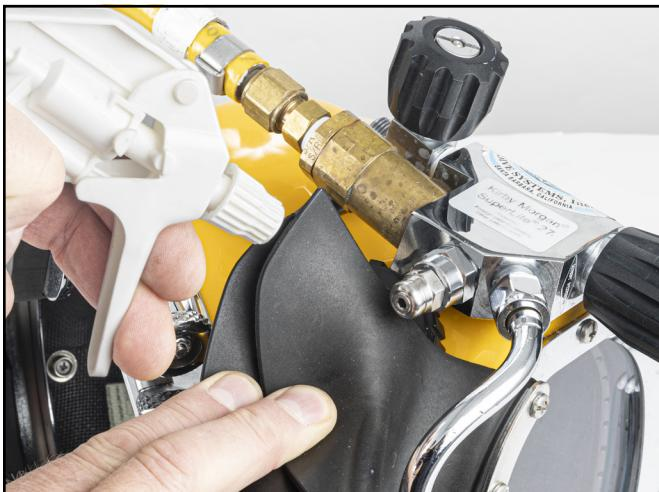
5. Open divers' umbilical gas supply valve on the console, then slowly increase the umbilical pressure using the hand-loader/regulator on the
