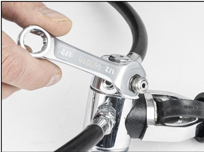
3. Remove, cut, and discard the overpressure relief valve body O-ring.
